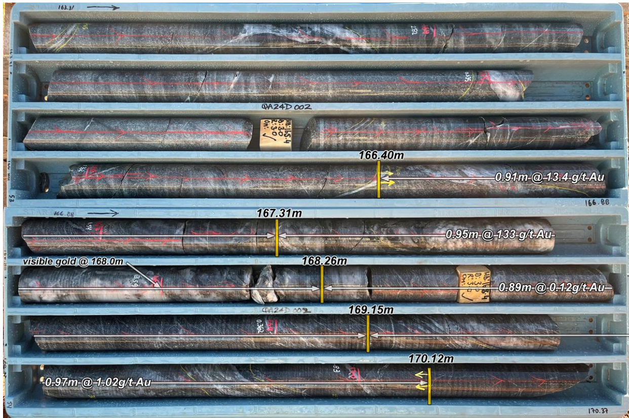
Figure 2: QA24D002 core tray showing visible gold intersection and the surrounding mineralisation
